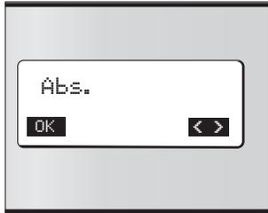
Press the arrow keys to change the setting to "Rel.". Then press the confirmation key.
