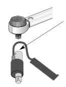
Place the square drive of the wrench into female socket side of the SMX.
